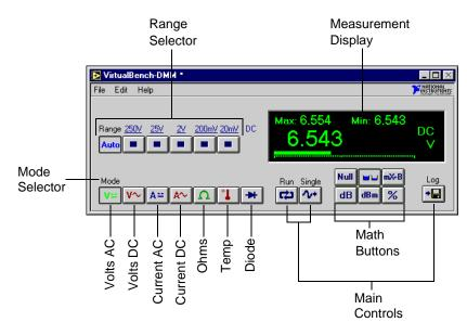
The front panel of VirtualBench-DMM has the following features:
